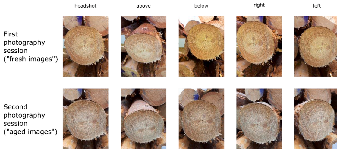
Fig. 2. Illustration of the photography scheme used in data collection. There was a time difference of five days between the first and second photography sessions. All images here depict the same log.
