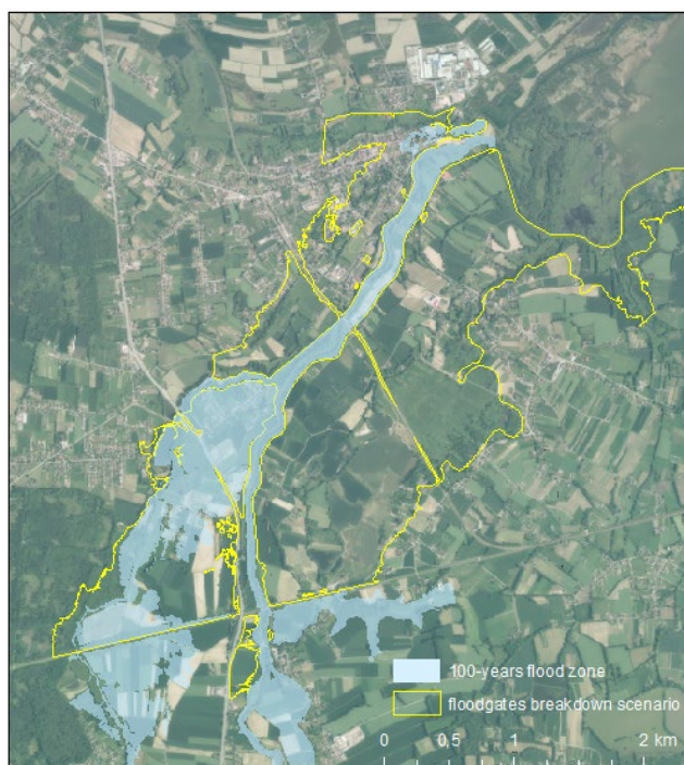
Figure 4. Illustration of the selected flood maps content: 100- years flood zone and the extent of floodgates breakdown scenario.
